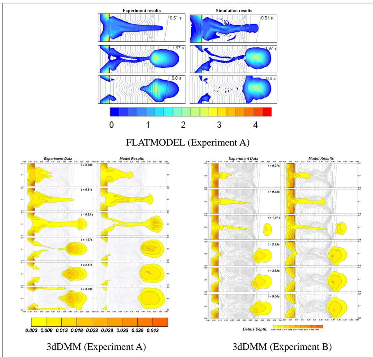
Figure 3: Simulation results by various models for the USGS flume test
