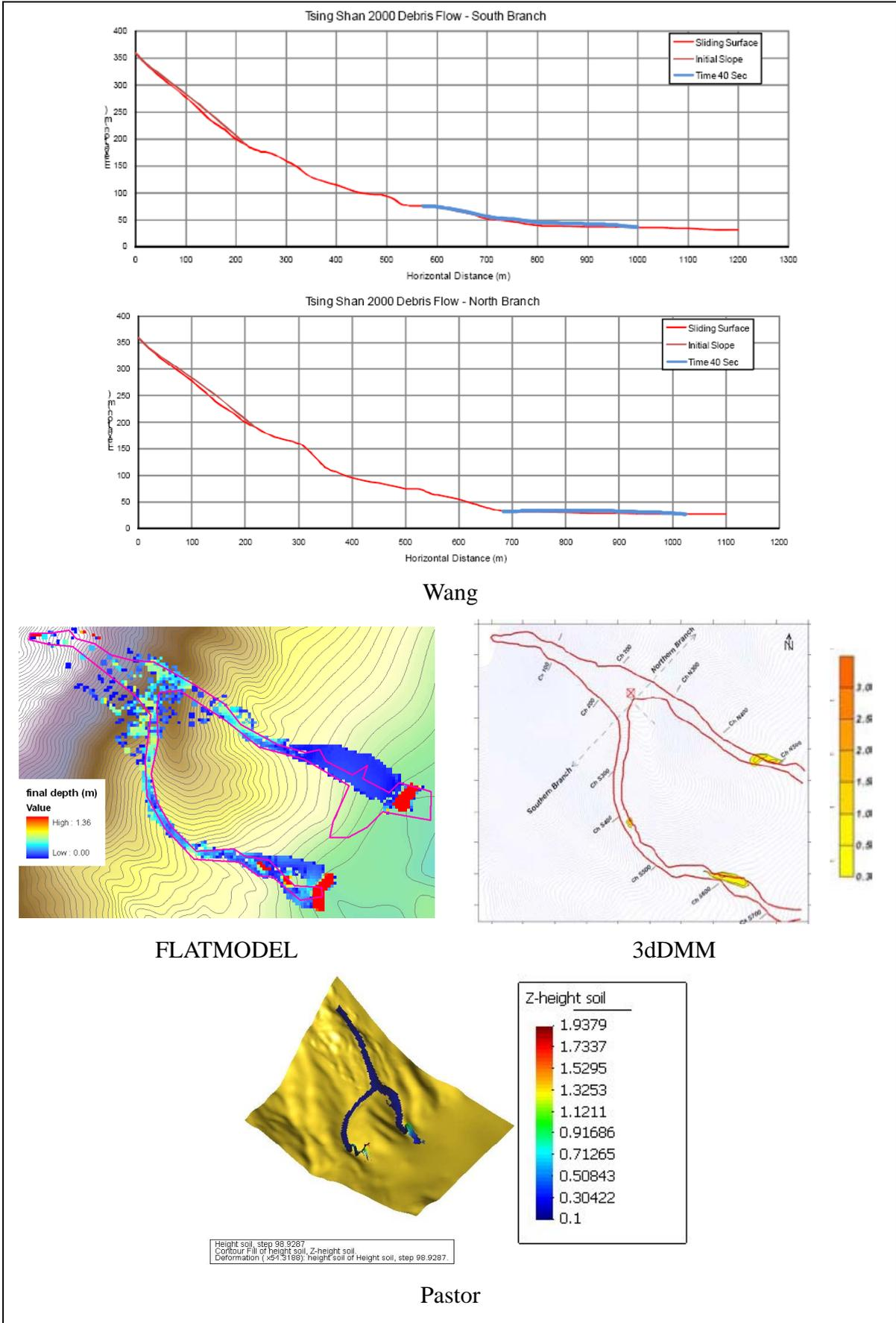
Figure 11: Simulation results by various models for 2000 Tsing Shan debris flow
