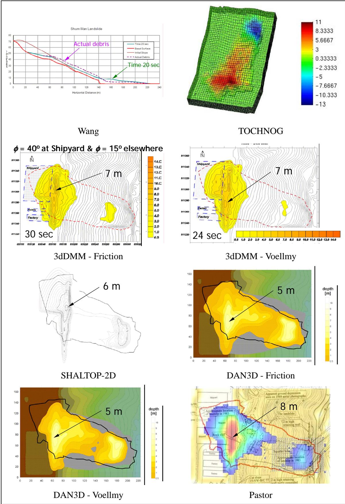
Figure 7: Simulation results by various models for Shum Wan landslide
