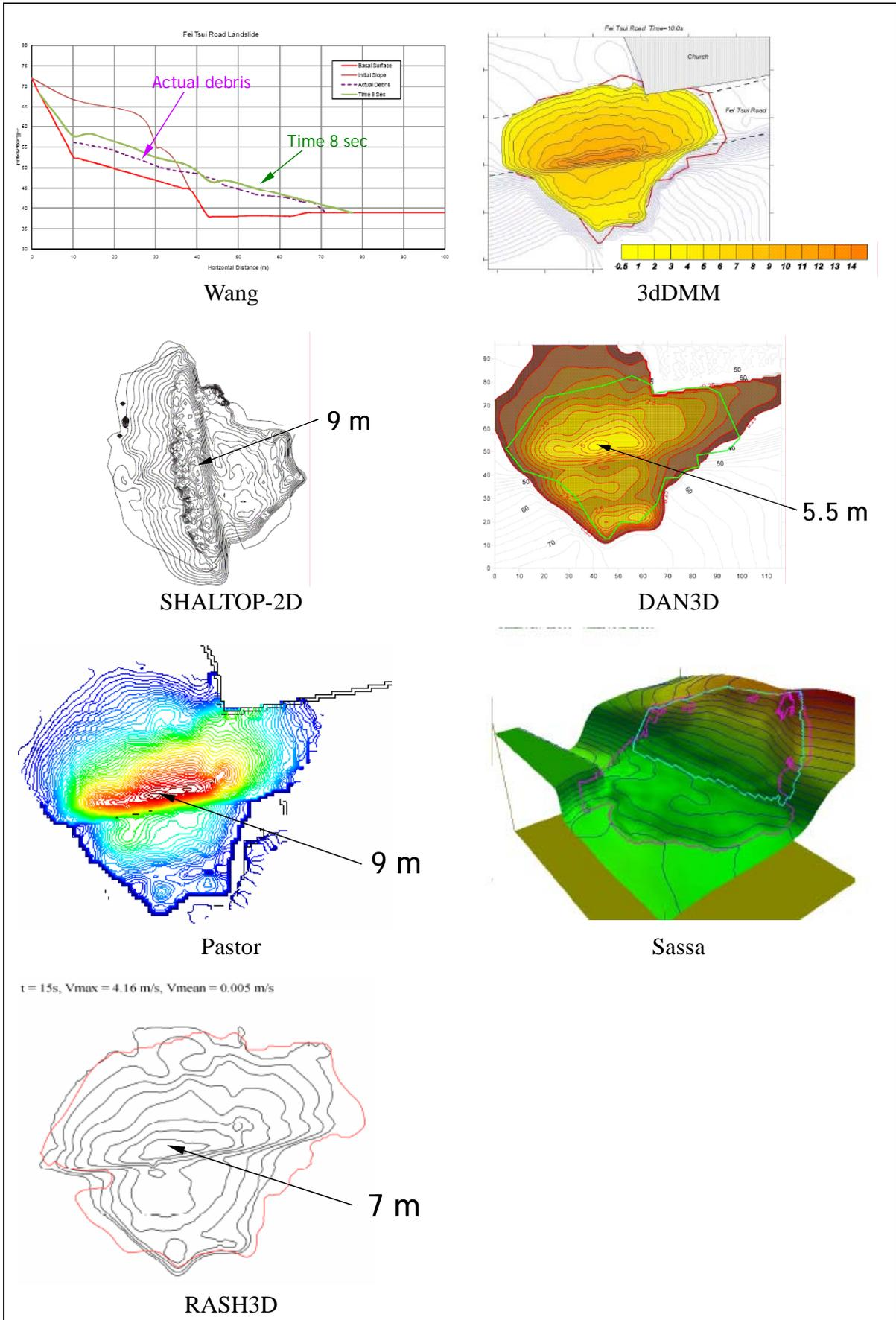
Figure 6: Simulation results by various models for Fei Tsui Road landslide
