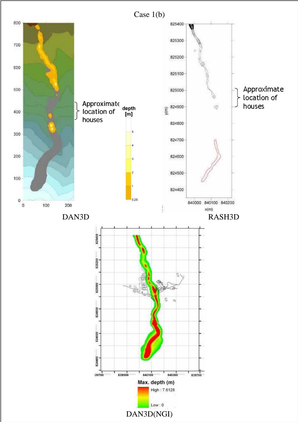
Figure 5(b) (Con't): Simulation results by various models for Tate's Cairn landslide forward prediction
