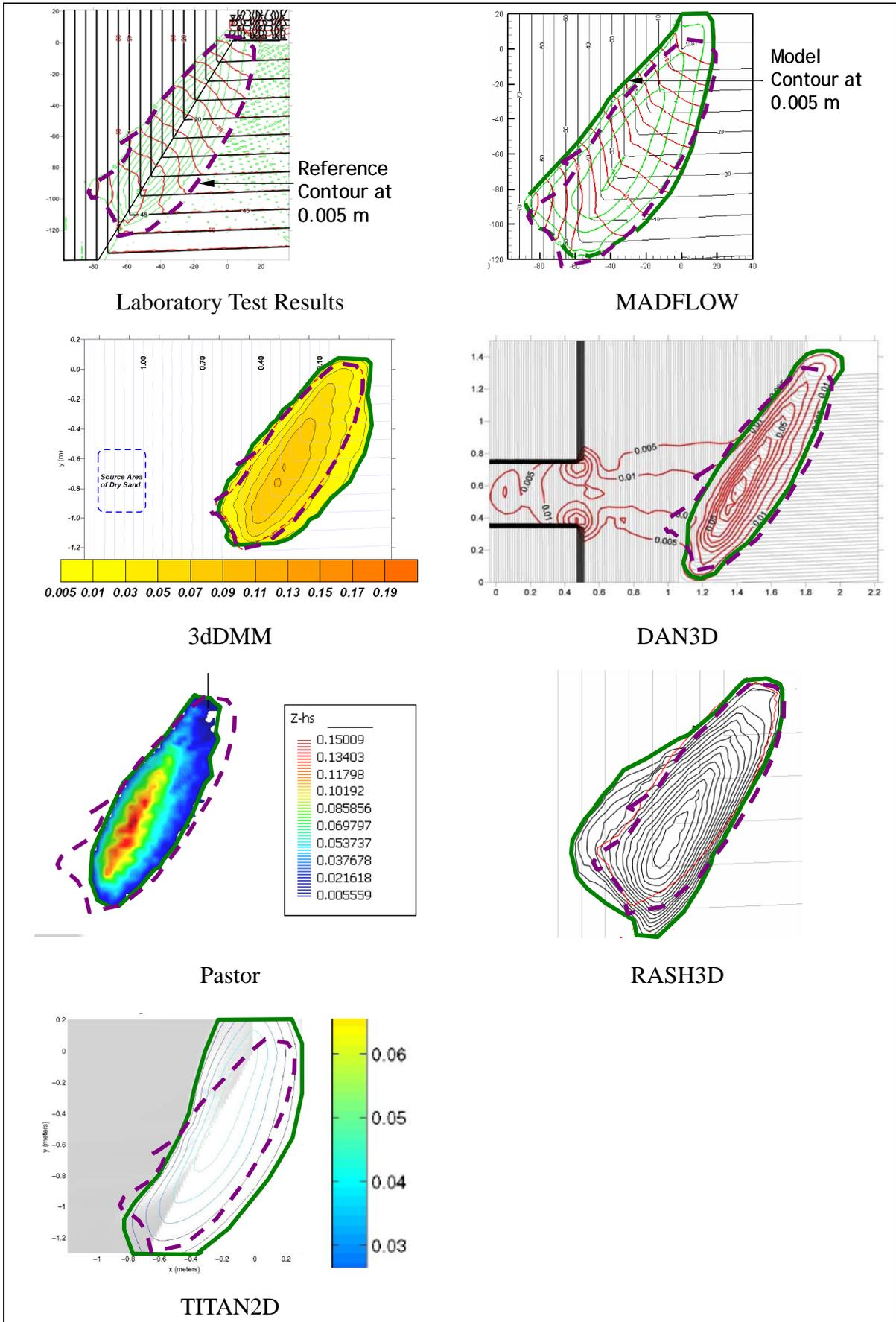
Figure 2: Simulation results by various models for the deflected sand flow experiment
