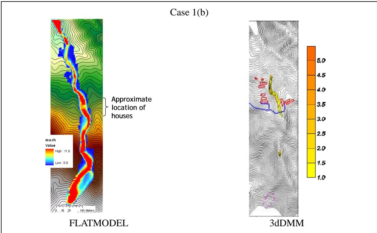
Figure 5(b): Simulation results by various models for Tate's Cairn landslide forward prediction
