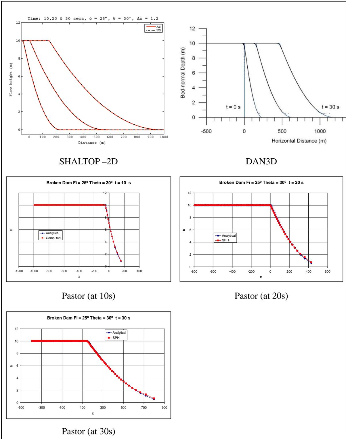
Figure 1 (Con't): Simulation results by various models for the dam break scenario
