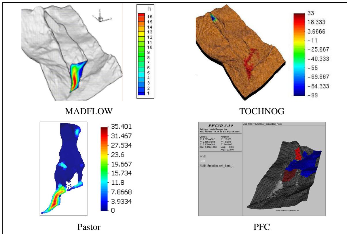
Figure 12: Simulation results by various models for Thurwieser rock avalanche
