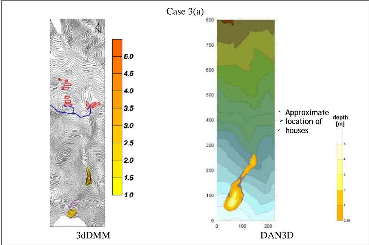
Figure 5(a) (Con't): Simulation results by various models for Tate's Cairn landslide forward prediction
