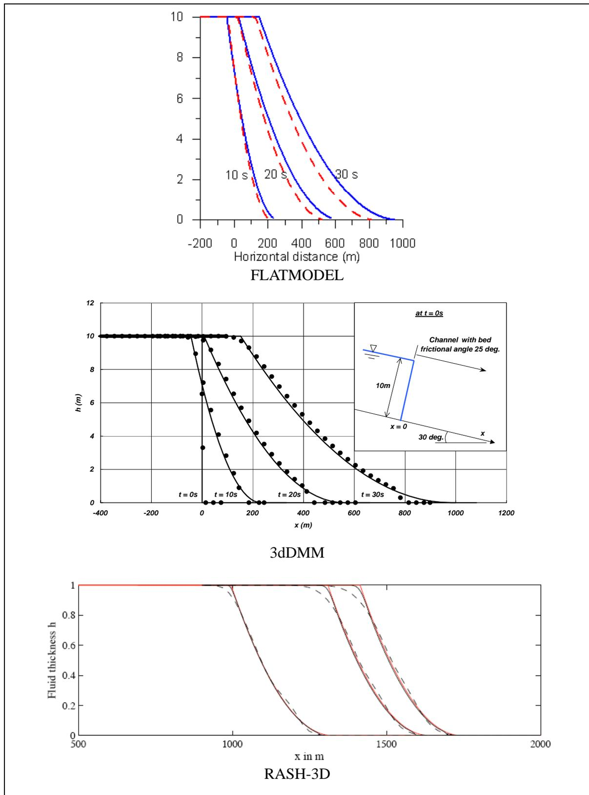
Figure 1: Simulation results by various models for the dam break scenario
