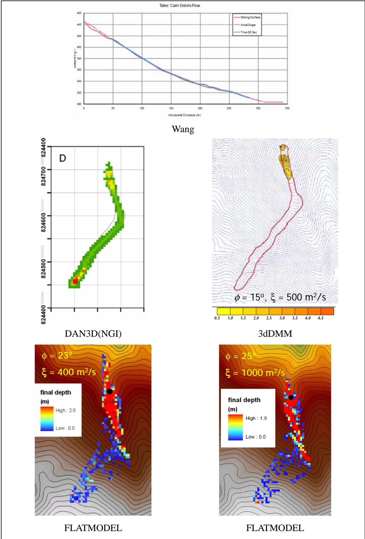
Figure 4: Simulation results by various models for Tate's Cairn landslide
