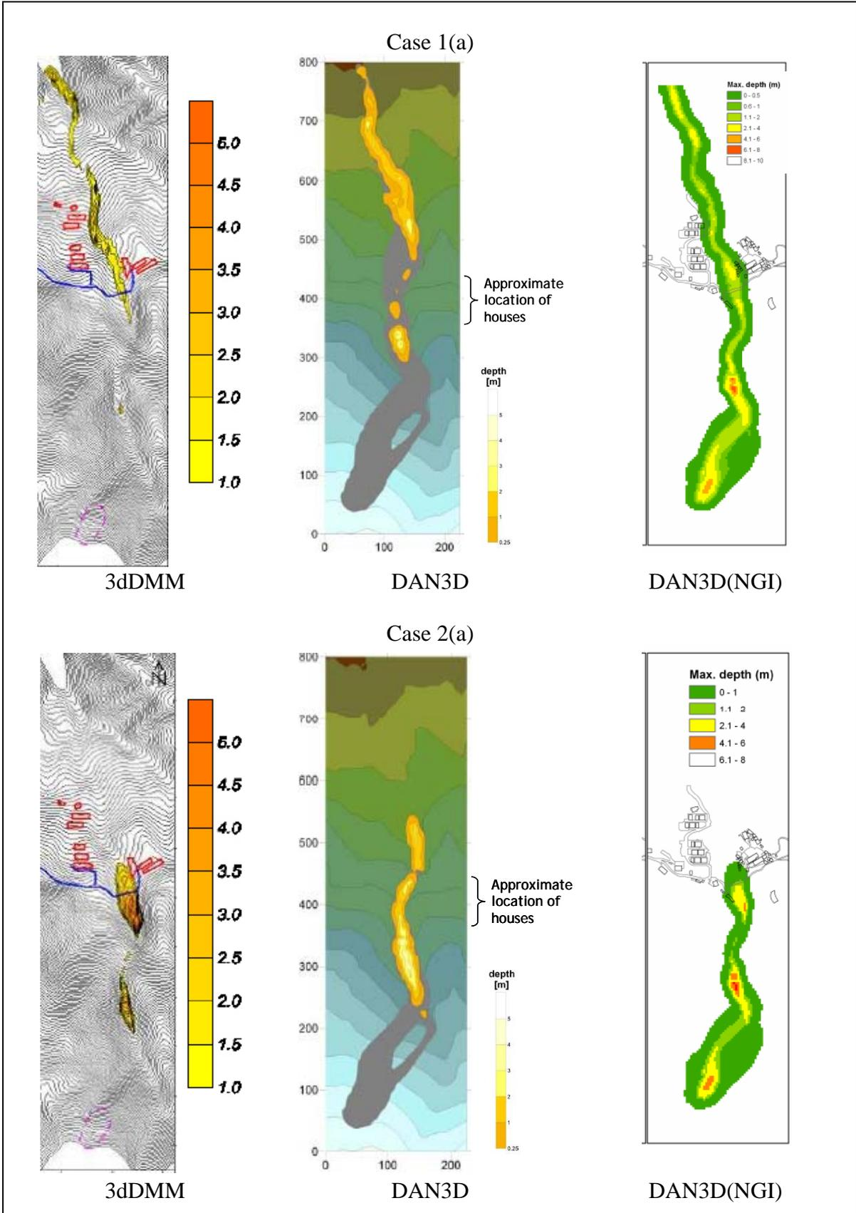
Figure 5(a): Simulation results by various models for Tate's Cairn landslide forward prediction
