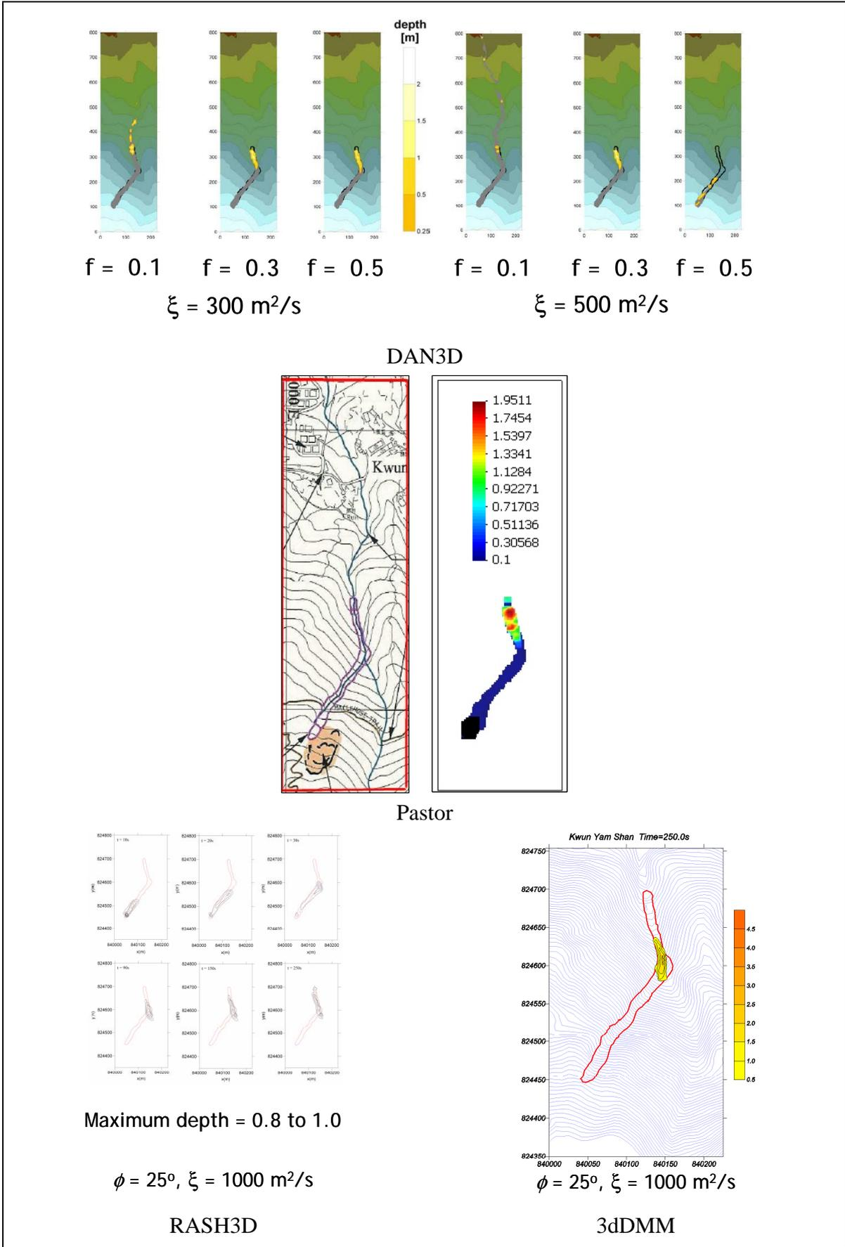
Figure 4 (Con't): Simulation results by various models for Tate's Cairn landslide
