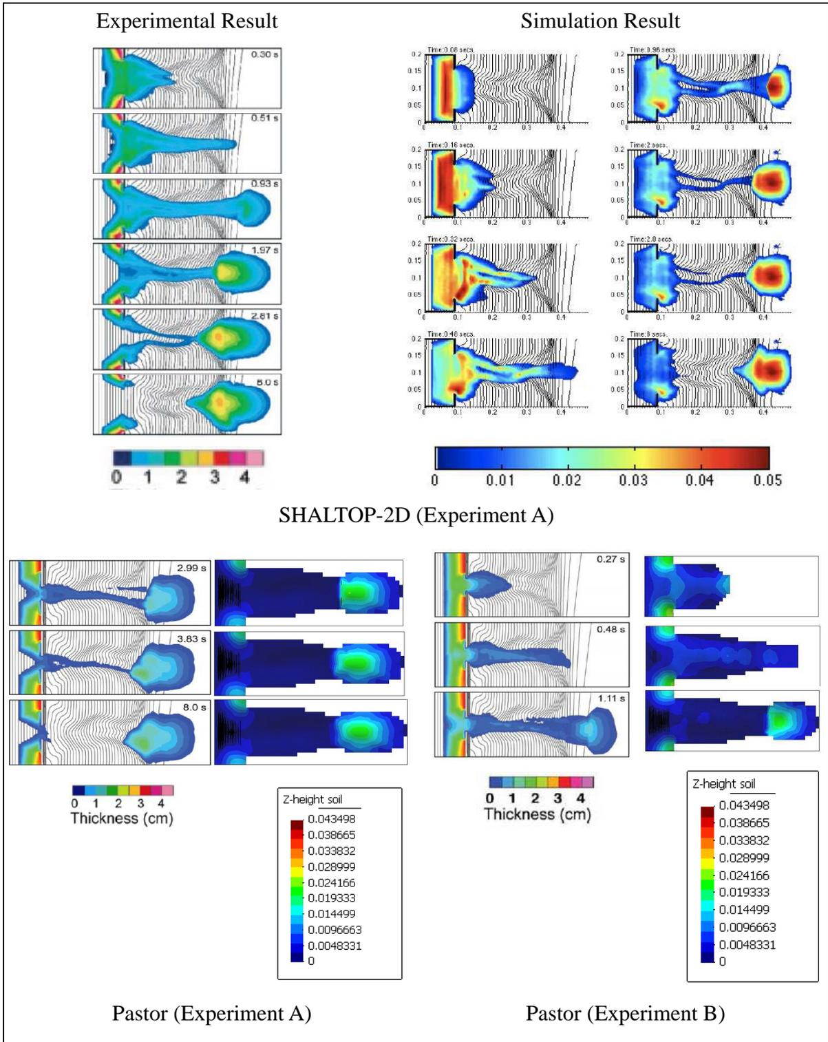
Figure 3 (Con't): Simulation results by various models for the USGS flume test
