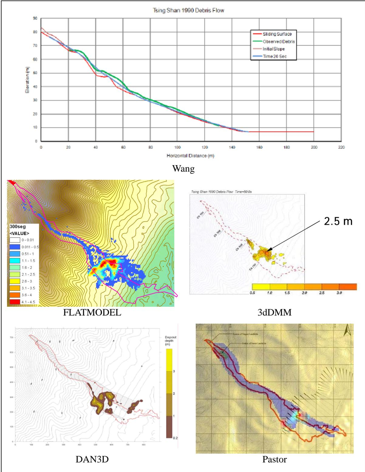
Figure 10: Simulation results by various models for 1990 Tsing Shan debris flow
